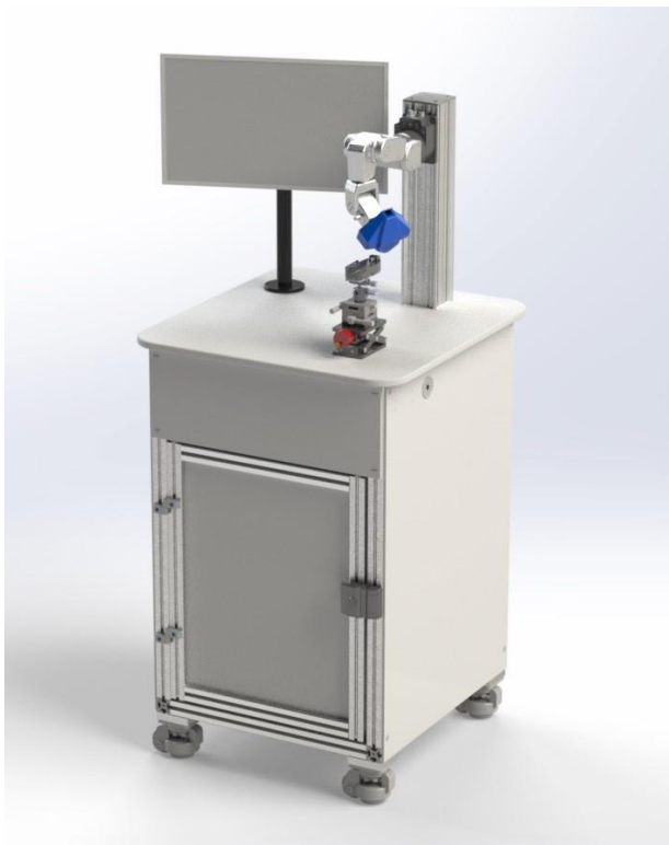
Figure 2: Rendering of the HaloC 375 complete system on a mobile cart, where the imaging head is mounted to a robotic art support, which enables freeform three-dimensional imaging. Cart height: 110 cm; width: 65 cm; depth: 65 cm.
