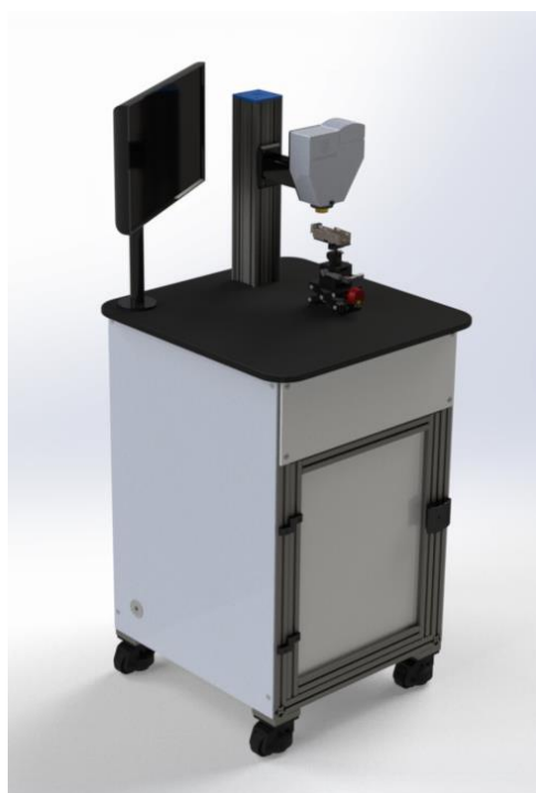
Figure 2: Rendering of the Halo 375 complete system on a mobile cart, where the imaging head is mounted vertically. Cart height: 110 cm; width: 65 cm; depth: 65 cm.
